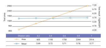
Result is accurate and stable, not affected by the dilution ratio and sample sedimentation
