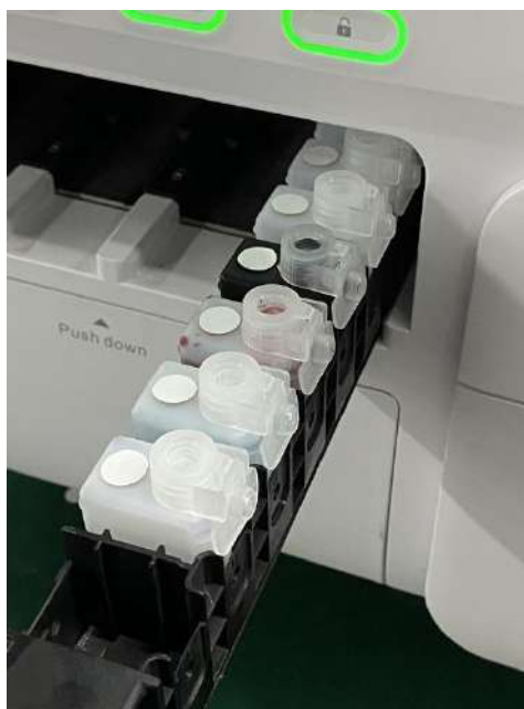
Figure 6-3 Uncover the reagent bottle and fasten it between two clamping side walls
