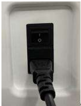
Figure 2-1 Power Cable Connection
