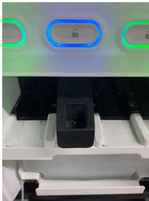
Figure 6-4 Properly install the reagent rack
