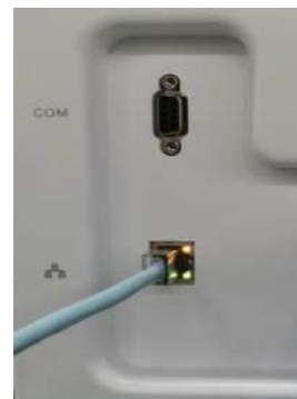
Figure 2-2 Data Cable Connection
